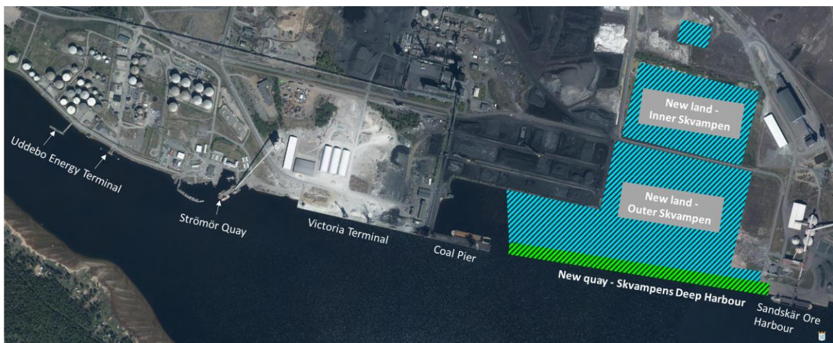
Figure 3. Malmporten Project - infill areas and the new deep harbour
