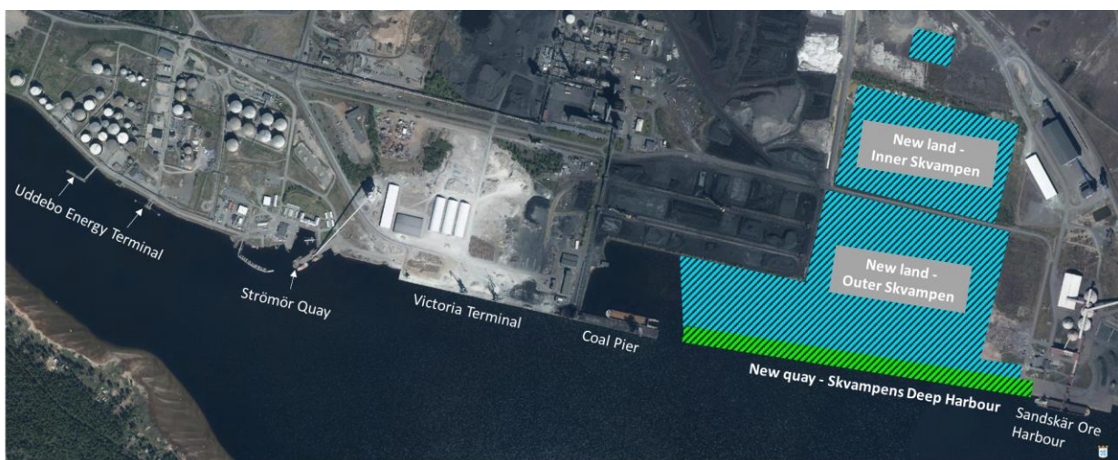
Figure 3. The Malmporten Project - infill areas and the new deep harbour
